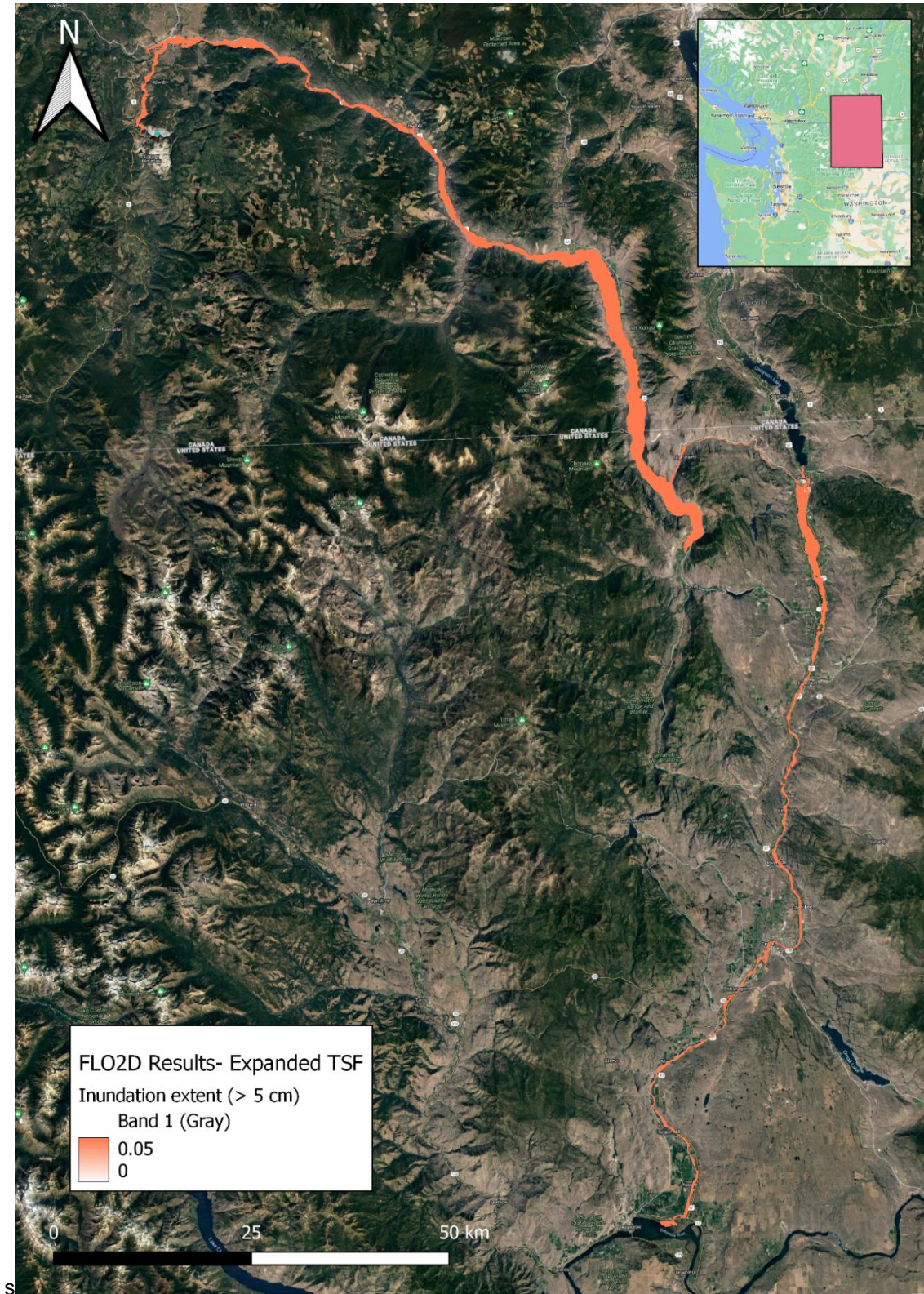
Figure 4-6: Inundation extent (> 5 cm depth) for the 40% breach, 12 hour duration scenario of the expanded TSF at CMM. 50 m spatial resolution, 480 hour simulation run time. CMM TSF is located in the upper left hand quadrant of the map, as illustrated in Figure A 20.
